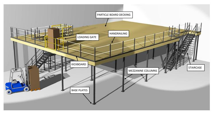
Important information required is the length, width and height of the floor as well as the number the staircases and amount of handrailing and gates required. Loading capacity of the structure should also be an important consideration depending on whether it is light, medium or heavy storage.
